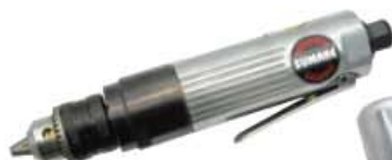
ST-4439 ST-4439C W/Keyless chuck 3/8" Air Straight Drill Speed: 4,500 rpm
