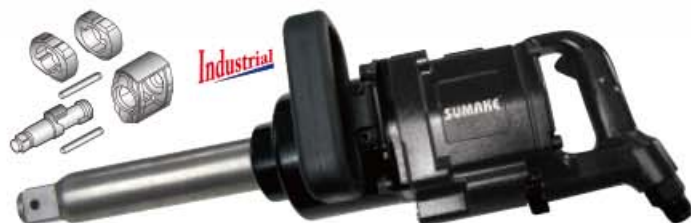
ST-5597 1-1/2" Dr. ST-5597-6 1-1/2" Dr. W/6" Ext. Anvil ST-5597-8 1-1/2" Dr. W/8" Ext. Anvil Twin Hammer Torque: 4,878Nm (3,600 ft-lb)
