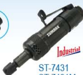
ST-7431G 1/4" ST-7431GM 6mm (Rotary Type) 0.45HP
