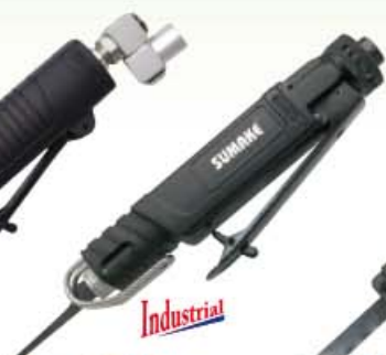
ST-66007 Mini Air Body Saw Vibration Reduction W/18T, 24T, 32T Blade (Alum. Housing) Speed: 11,000 bpm
