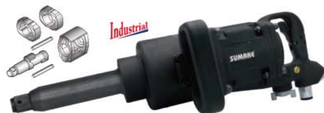
ST-5598 1" Dr. ST-5598-6 1" Dr. W/6" Ext. Anvil ST-5598-8 1" Dr. W/8" Ext. Anvil Twin Hammer Torque: 4,342Nm (3,200 ft-lb)
